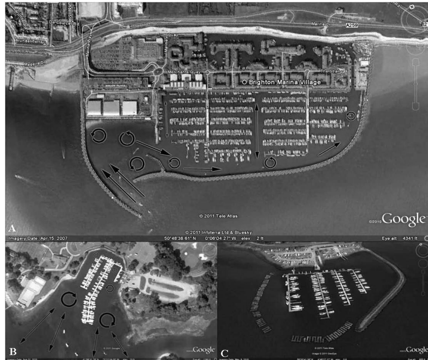
Figure 1: (A) Aerial view of the enclosed Brighton Marina. 220 Arrows illustrate limited water circulation and velocity resulting from the marina's enclosed design. Brighton Marina is the largest marina in the United Kingdom with 1600 yacht berths, accommodating vessels between five and twenty-five meters in length for short or long stays. 221 (B) Aerial view of the open Longshore Club Park and Country Club marina in Westport, Connecticut. Arrows illustrate the enhanced water circulation and velocity resulting from the marina's unenclosed design. 222 (C) Rhu Marina on the west coast of Scotland is made from prefabricated parts and is further sheltered by its own integral floating concrete breakwater system. 223
